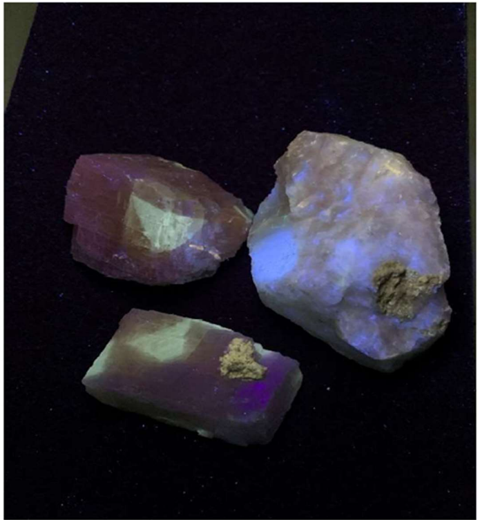
2 Calcite specimens under UV-C radiation. Cleavage sections about 50mm wide. New Point Stone St. Paul north pit, Indiana 2023
