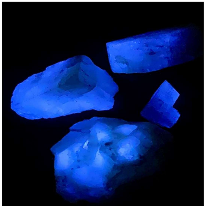
4 Calcite specimens after UV-C radiation (254nm), with Terlingua-type, blue/white phosphorescence response. Cleavage sections about 50 mm wide. New Point St. Paul plant north pit Indiana 2023
